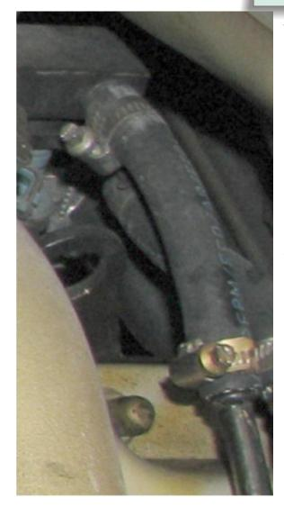
These are the rear high pressure fuel line hoses feeding the fuel rails. In the view at the left, note the top hose feeds the left side fuel rail and the bottom hose goes over to the right fuel rail.
