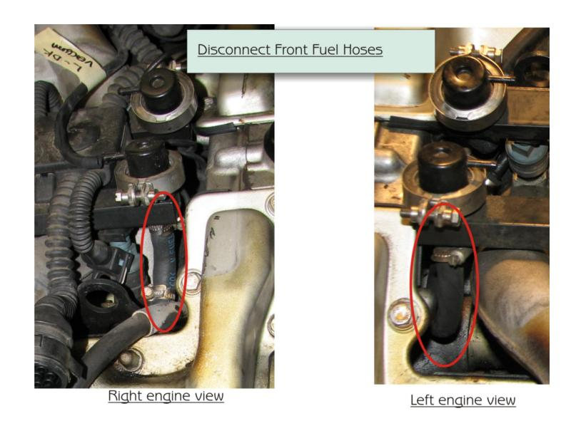
Front Fuel Lines - disconnect (Under Fuel Regulators)
