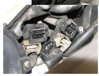
Pulse Sender/Cylinder ID connector Removal (Circled) This shows the location of the four 10 mm (socket) bolts that hold the connector retaining clips to the cylinder head. They're hard to see as they're covered in
