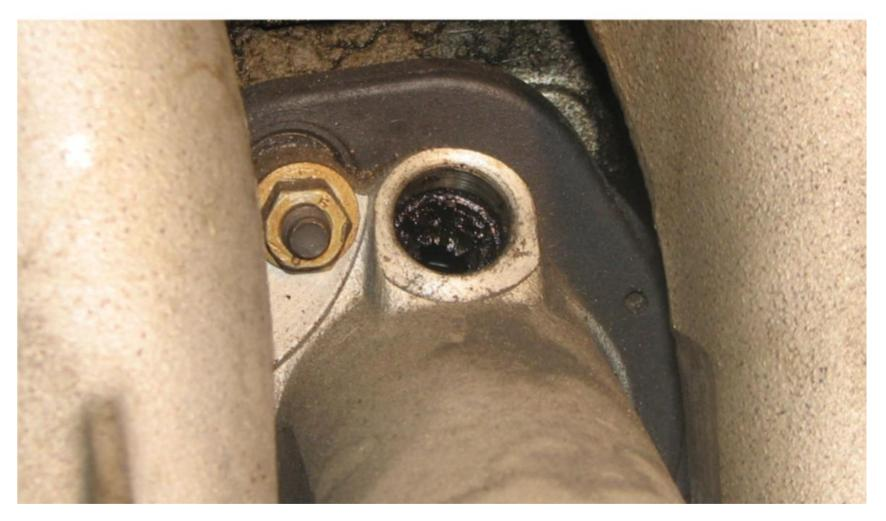
All of my injector ports were "sludged" up as the picture shows. I'm told this is normal when using nonsynthetic oil, but if synthetic is used, the sludge is reduced.
