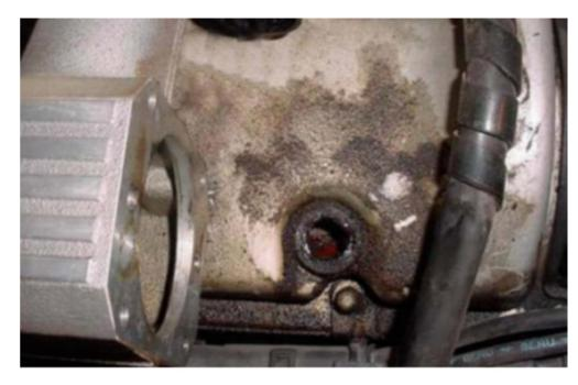
Remove the PCV valves by pulling them up and out of the rubber seals/grommets. Both of these seals will most likely need to be replaced on your engine as they typically have hardened and leak.
