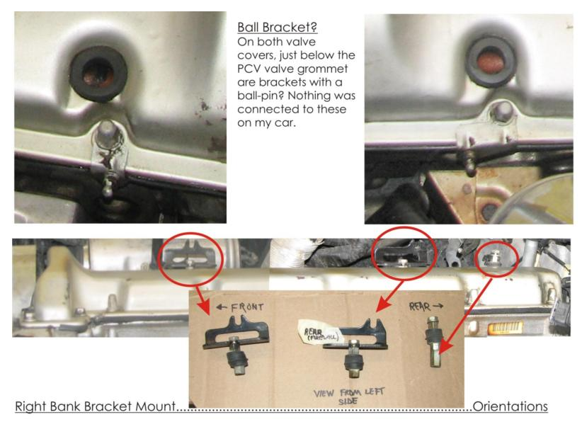
Note the stand-off/extension on the hard fuel line mount on the far right.
