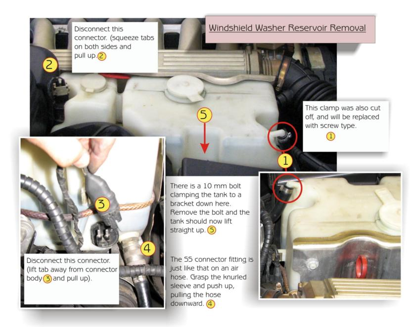
DisconrectPowe washer tank out of the way . I left the braided hose attached to the tank.
