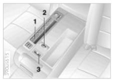
In order to operate certain functions from the rear passenger area as well, the corresponding controls are integrated in the center armrest.
