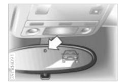
The semisolid reacts chemically to this electrical current, thus providing dimming of the mirror through an infinitely-variable range (electrochromic technology).
