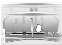
The hazard warning triangle is readily accessible. It is stored in the container for the onboard tool kit mounted in the luggage compartment lid.
