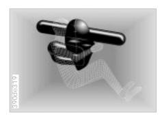
Deceleration sensors continuously monitor the physical forces acting upon the vehicle. If, as the result of a frontal collision, a deceleration is reached at which the protection of the safety belts alone is no longer adequate, the gas generators of the driver and passenger-front airbags are ignited. However, the passenger-side airbag is only triggered if an additional sensor has recognized that the passenger seat is occupied.
