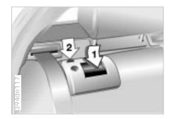
The rear backrest is divided into two sections, one-third and two-thirds of the seat respectively. For carrying longer objects, you can fold down either section of the backrest separately.
