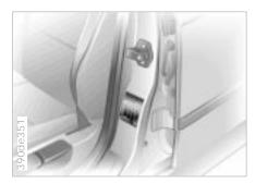
The inflation pressures are indicated on a label attached to the B-pillar behind the driver's door (visible with door open).
