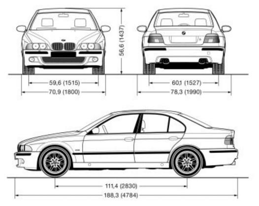
All dimensions are given in inches (mm). Minimum turning circle dia.: 38.1 ft (11.6 m)
