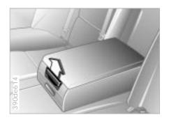
Fold the armrest out and open the cover by lifting the handle (arrow).
