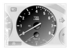
The orange early warning zone appears depending upon the engine temperature. As the engine temperature increases, more and more sectors of this early warning zone disappear.
