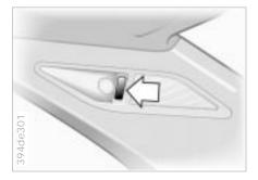
The reading lamps are located in the front near the interior lamp. There are also reading lamps in the rear. They can be switched on and off with the switch (arrow) next to each lamp.
