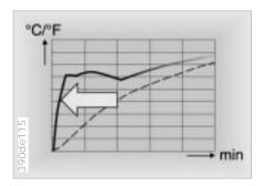
The latent heat storage system accumulates and stores engine heat – even for several days at extremely low outside temperatures. After the engine is started, this accumulated heat can be utilized immediately to defrost the windshield and side windows and to remove condensation from them. In addition, the time required for warming the interior of the vehicle and for warming up the engine (arrow) are significantly reduced.
