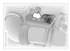
4 Start by connecting the jumper cable from the positive terminal of the support vehicle to the positive terminal connector located in your BMW's engine compartment. The cover of the auxiliary terminal for jump starting is identified with a "Batt. +" sign. Refer to the illustration. Remove by lifting the cap.
