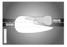
Xenon lamps illuminate the side and front areas of the vehicle with significantly more brightness and uniformity than traditional halogen lamps.
