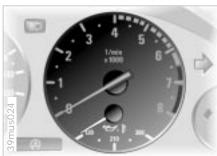
The normal operating temperature is in a range between +176 °F (+80 °C) and +248 °F (+120 °C). Do not exceed the maximum temperature of +302 °F (+150 °C).
