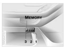
You can store and call up three different seat, exterior mirror and steering wheel positions. The illustration shows the buttons on the driver's door, for making these position adjustments.
