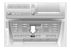
Whenever it is required, this system changes the settings of the Servotronic power steering, and the accelerator pedal response from a performance-comfort mode to a pure performance mode. That is, steering response becomes more performance-oriented and the response of the accelerator pedal is much more spontaneous (Performance Recognition).
