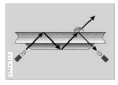
The rain sensor controls windshield wiper operation, depending on how wet the windshield is.
