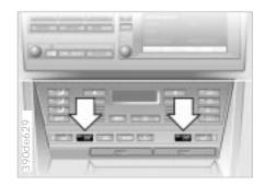
Active changes in the seat's surface help to avoid muscle cramps, pain in the spine's lumbar region and fatigue. To activate the seat, press the button (arrow).
