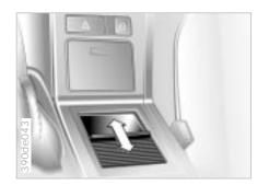
The cover of the storage compartment on the inclined surface of the center console can be pushed open or closed (arrow). If your vehicle is equipped with a cassette holder\*, open each cassette compartment by pressing the small button.
