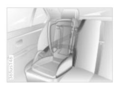
All of the rear belt retractors and the front passenger's safety belt can be locked for mounting and securing child restraint systems.
