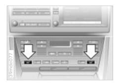
The seat cushion and backrest can be heated when the ignition key is in position 2. You can call up different heating modes by repeatedly pressing the keys.
