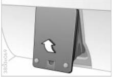
4 Use the magnetic retainers to attach the cover panel to the upper surface (metal surface below rear tray) of the luggage compartment.
