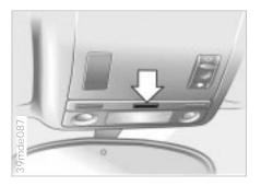
The interior lamps operate automatically.
