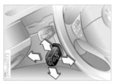
The steering wheel can be moved in any of four directions. Adjust by moving the control lever in the desired direction.
