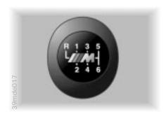
The shift lever's neutral gate is located between 3rd and 4th gears.
