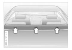
If you use a child restraint system with a tether strap, three additional tether anchorage points have been provided (refer to the arrows in the illustration). Depending on the location selected for seating in the rear passenger area, attach the strap hook to the corresponding anchorage point to secure the child restraint system.
