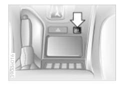
Use this button to operate the central locking system when the front doors are closed. The doors and luggage compartment lid are unlocked or locked only. The antitheft alarm system is not activated. Also, the fuel filler door remains unlocked to allow refueling.
