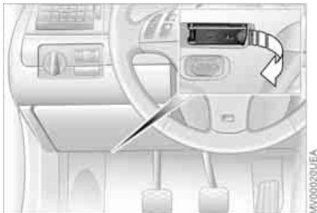
The Onboard Diagnostic OBD interface socket is located on the left of the driver's side under the instrument panel and under a cover.
