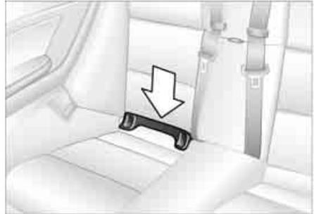
The LATCH anchorage points are identified by symbols.
