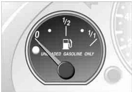
Once the indicator lamp stays on continuously, there are still approx. 2 gallons/8 liters of fuel in the fuel tank. Fuel tank capacity approx. 16.6 gal./63 liters.
