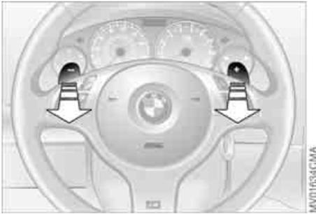
Shifting gears with shift paddles on steering wheel:
