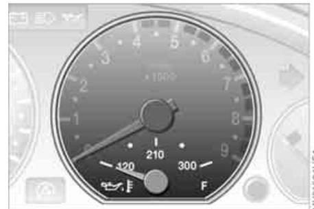
The general operating temperature lies between 175 °F/80 °C and 250 °F/120 °C. During high-performance driving, do not exceed a maximum value of 300 °F/150 °C.
