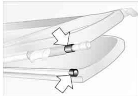
2. Flip out both sides and lock into place. It is essential for the two components marked in the illustration to mesh at this point
