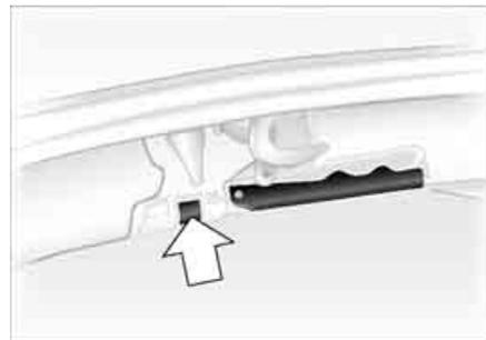
4. Open the two front locking levers on the hardtop. Press on the buttons to do so. The levers will release slightly. Open the levers as far as possible
