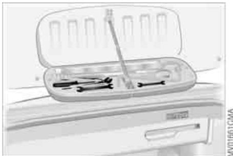
The onboard tool kit is located in the luggage compartment lid.
