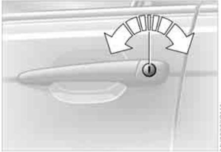
Turning the key in the door lock once unlocks the driver's door, the fuel filler door and the glove compartment.
