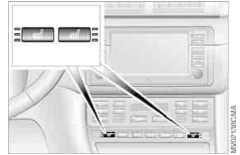
The seat cushion and backrest can be heated with the ignition key in position 2.
