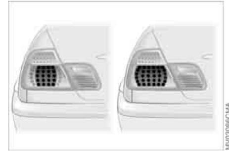
Brake force display indicates to the road users behind you how hard you are braking.
