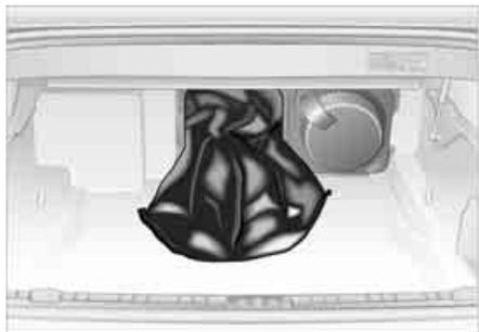
5. Secure the cover panel with the magnetic retainer on the rear wall, then pull out the ski bag.
