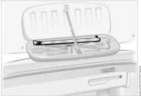
The hazard warning triangle is stored ready to use in the luggage compartment lid inside the toolbox for the onboard tool kit.
