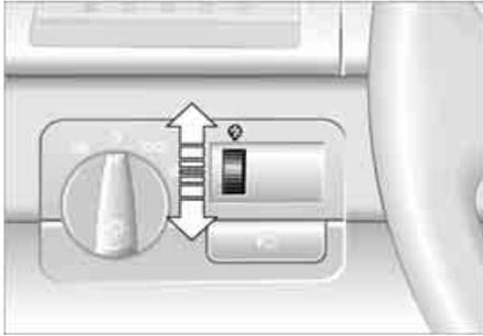
Turn the rotary dial to control the lighting when the parking or low beam lamps are on.
