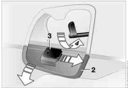
5. Before installing, first flip down the cover panels 2 that are located underneath the left and right interior lamps. To do this, press on the slight bump on cover panel 2. There is a holder in the cover panel to securely store the trim pieces that have been removed. Pull the adapter 3 out of the holder, clip the trim piece into the bottom and reinsert the adapter
