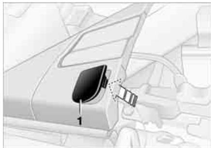
3. Press trim piece 1 on each side of the car upwards and remove. Do so by pulling the tab on trim piece 1 in the direction of travel
