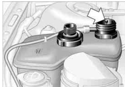
**Checking the coolant level**
