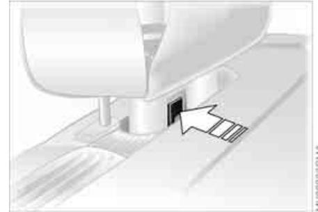
If, after being automatically triggered, the protective function is not needed, then the rollover protection system can be lowered back into place. No special tool is needed for this.
