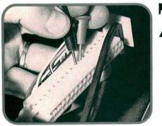
At first glance, it looks like you'll have to do all of your ECU harness connector testing with the ECU disconnected unless you've got a dedicated breakout harness. The plastic cover at the back of the connector can be removed if you're especially persistent. This reveals the back of the ECU connector's terminals.
