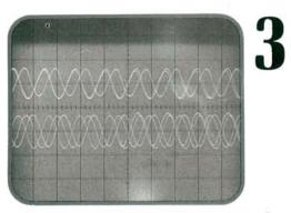
It's hard to see the flywheel teeth without removing the transmission. An oscilloscope can be used to quickly check the teeth for damage. Backprobe the RPM sensor's yellow lead wire, then attach the oscilloscope's probe. A good flywheel will have a smooth, even wave pattern. Damaged teeth will show up as a skip in the pattern.
