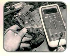
An off-idle hesitation and other driveability problems can be caused by water in the throttle switch. The water can bridge the idle contacts, which makes the ECU think the engine is idling, even after the throttle is opened. The switch isn't waterproof, and can be damaged if the engine is steam cleaned.
