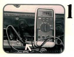
The RPM and Mark Sensor signals are probably the two most important Motronic input sensors. Internal resistance for both sensors should be between 800 and 1250 ohms. ECU bias voltage to the sensors should be between 1.0 and 2.5 volts. Also check for shorts between the sensor wiring and the harness shielding.
