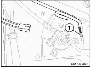
Splice the wire ends together, solder the connection and insulate it with shrink-wrap tubing (1).
