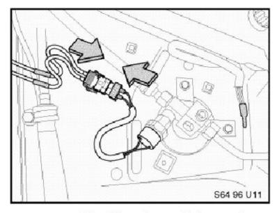
3.4 Install the service port quick-disconnect adapters.
