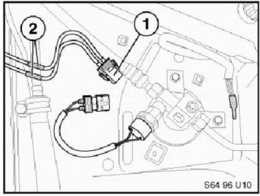
Strip the isolation from the wire ends and install a new black 2-pin connector (1), repair set D, P/N 1 378 400. Splice the wire ends of the new connector together with the wire ends from the harness, solder the connections and insulate it with shrink-wrap tubing (2).
