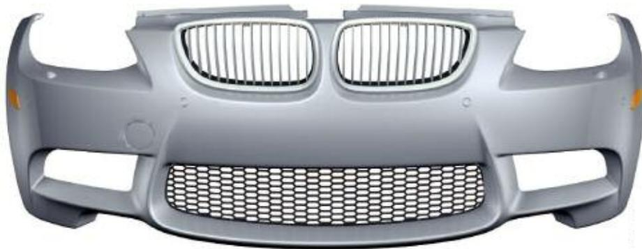
Front bi-xenon headlamp units are identical to the series E92. The M3 front bumper overhang is longer than that of the series E92.
