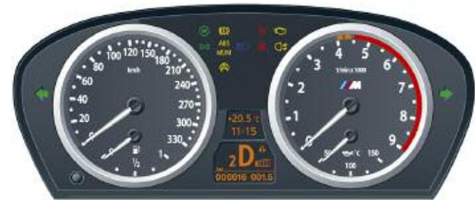
This conveys a unique, almost race-car like ambience. Arranged between the two circular gauges are the displays for SMG mode, current gear and engine oil level.
