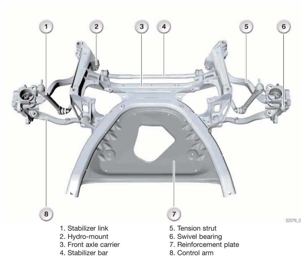
Axle alignment is performed at the tie rods. If necessary, the camber is corrected by removing the pin on the upper support bearing.
