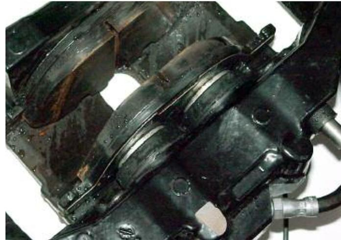
**Dual Piston Front Brake Caliper (close-up view)**
