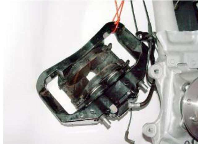
**Dual Piston Front Brake Caliper**
