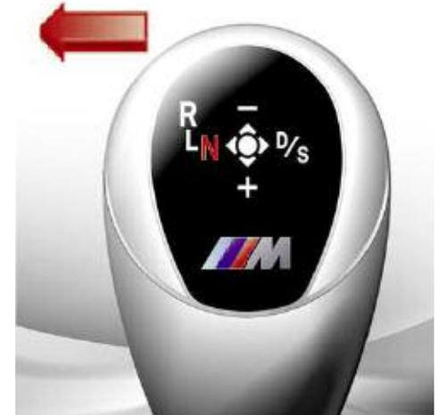
**Note: At the car wash, before stopping the engine you must deliberately shift to "N" and leave the transmitter in the ignition lock. (With Comfort Access it must remain in the car or be inserted in the ignition lock).**
