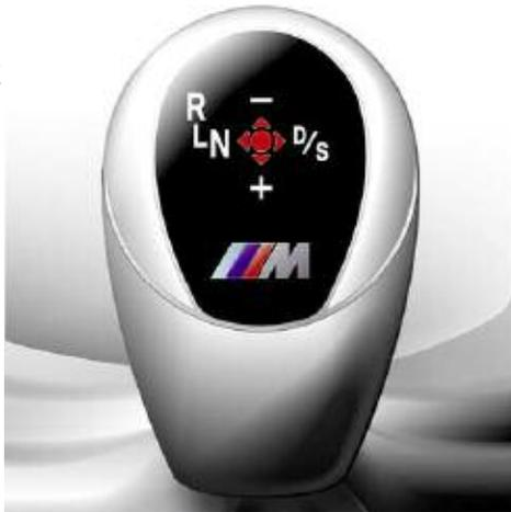
**M GWS selector lever during and after starting the engine**
