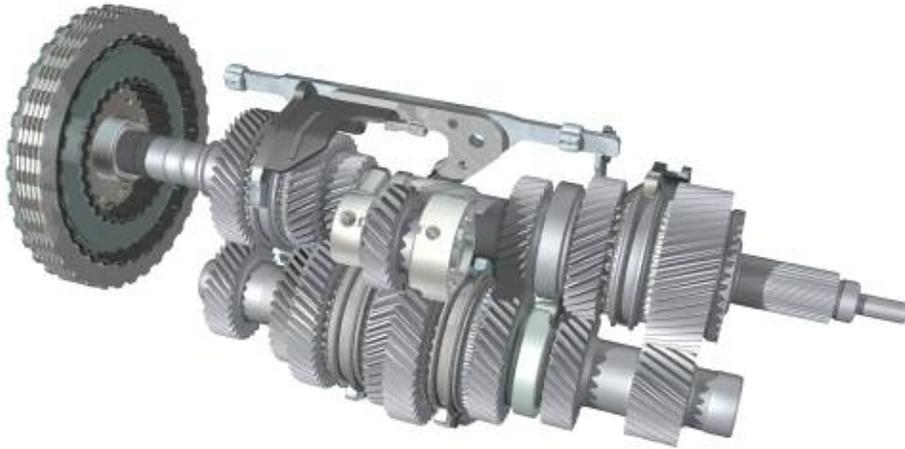
**M DCT sub-transmission 1 and sub-transmission 2 joined together with selector linkage**
