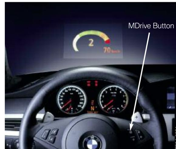
**Note:** If the indicator lamp flashes after pressing the button, then MDrive was unable to react, as the ABS Anti-lock Brake System or DSC Dynamic Stability Control is currently controlling the vehicle stability. Press the button again when the indicator lamp no longer flashes.
