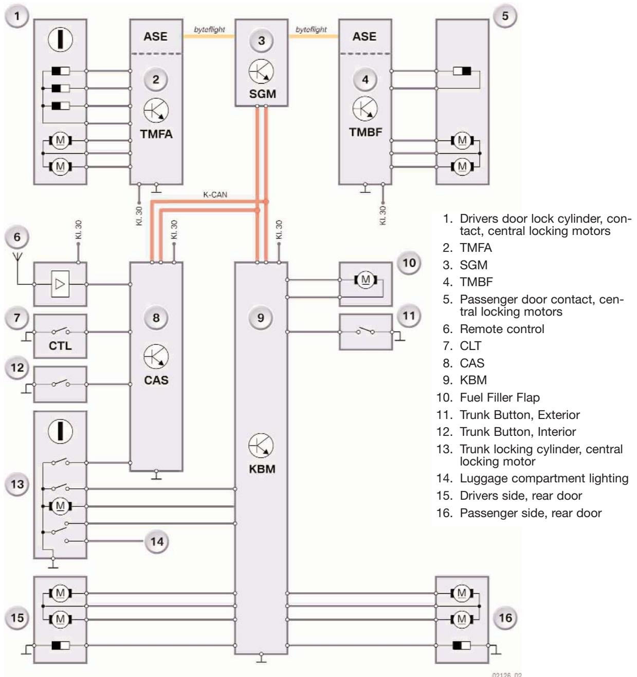
The central locking system consists of the following control points:
