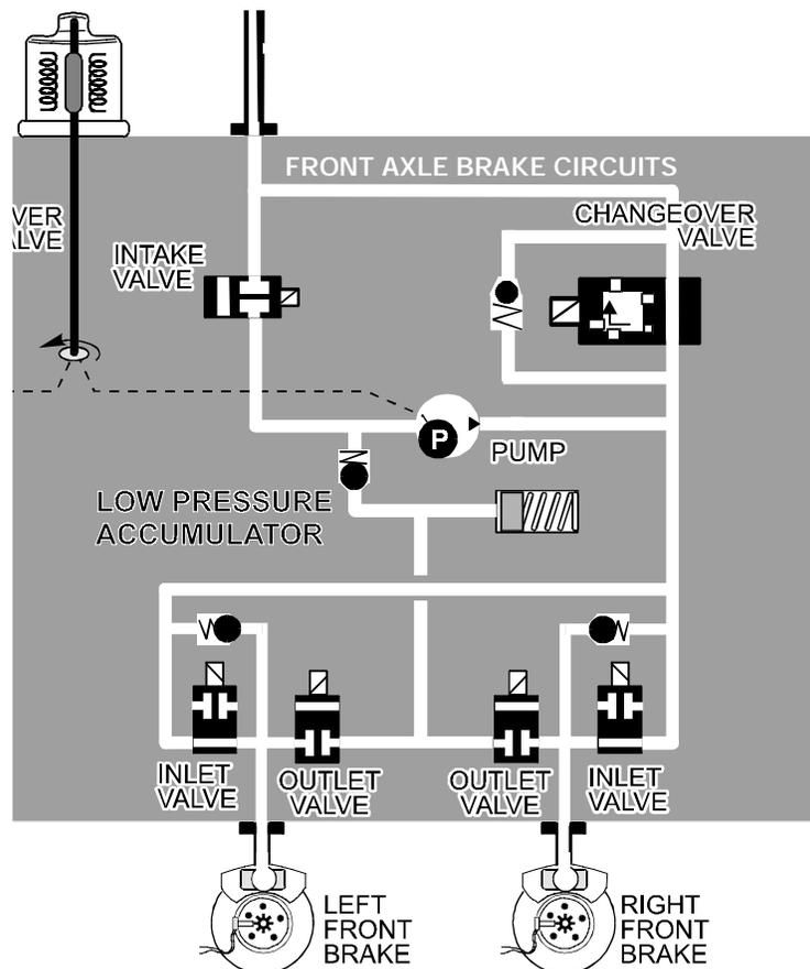
Pressure Release occurs when the control unit energizes the Outlet Valve while continuing to hold the Inlet Valve closed. The trapped brake fluid is released out of the calipers, reducing braking pressure.
