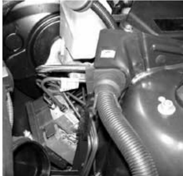
All processing functions for ABS, ASC or DSC are performed by the combined control unit/hydraulic unit. The MK 60 control unit is also responsible for processing the wheel speed signals and providing them to other control units.
