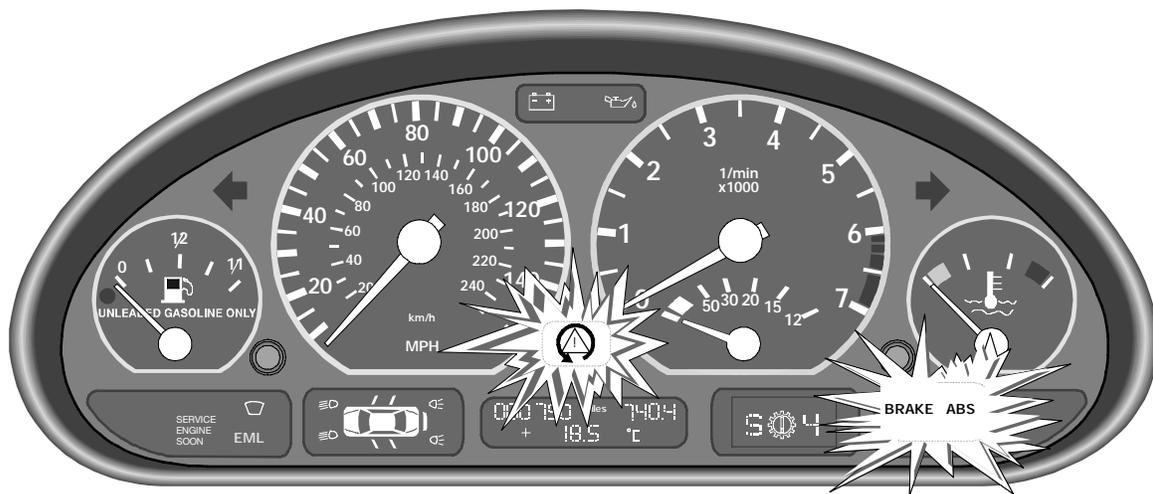
Three warning indicator lamps are arranged in the instrument cluster:
