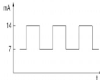
The sensor evaluation circuit is supplied 12V by the MK60 control unit. Output voltage from the sensor is approximately 10V. The control unit counts the high and low current pulses to determine the wheel speed signal.
