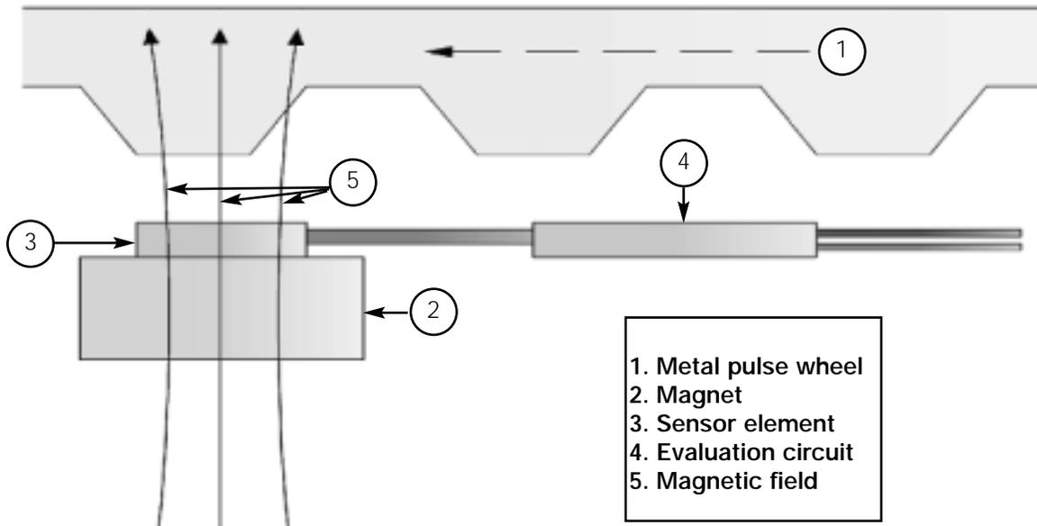
The sensor element is affected by the direction of the magnetic field, not the field strength. The field strength is not important as long as it is above a certain level. This allows the sensor to tolerate variations in the field strength caused by age, temperature or mechanical tolerances.
