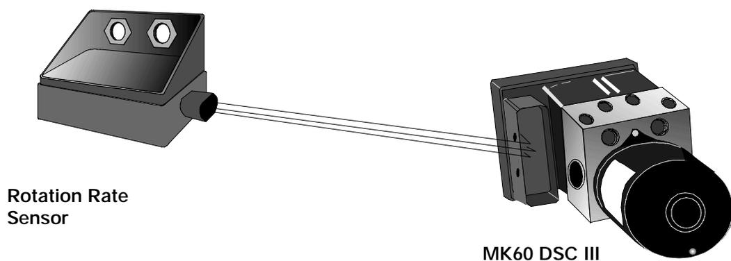
The MK60 DSC III for M.Y. 2002 incorporates a combined Rotation rate and Transverse Acceleration Sensor. The Sensor is connected to the MK60 control unit by the CAN bus. The Z3 version will retain separate sensors until the E36/7 is replaced by the E46/6.
