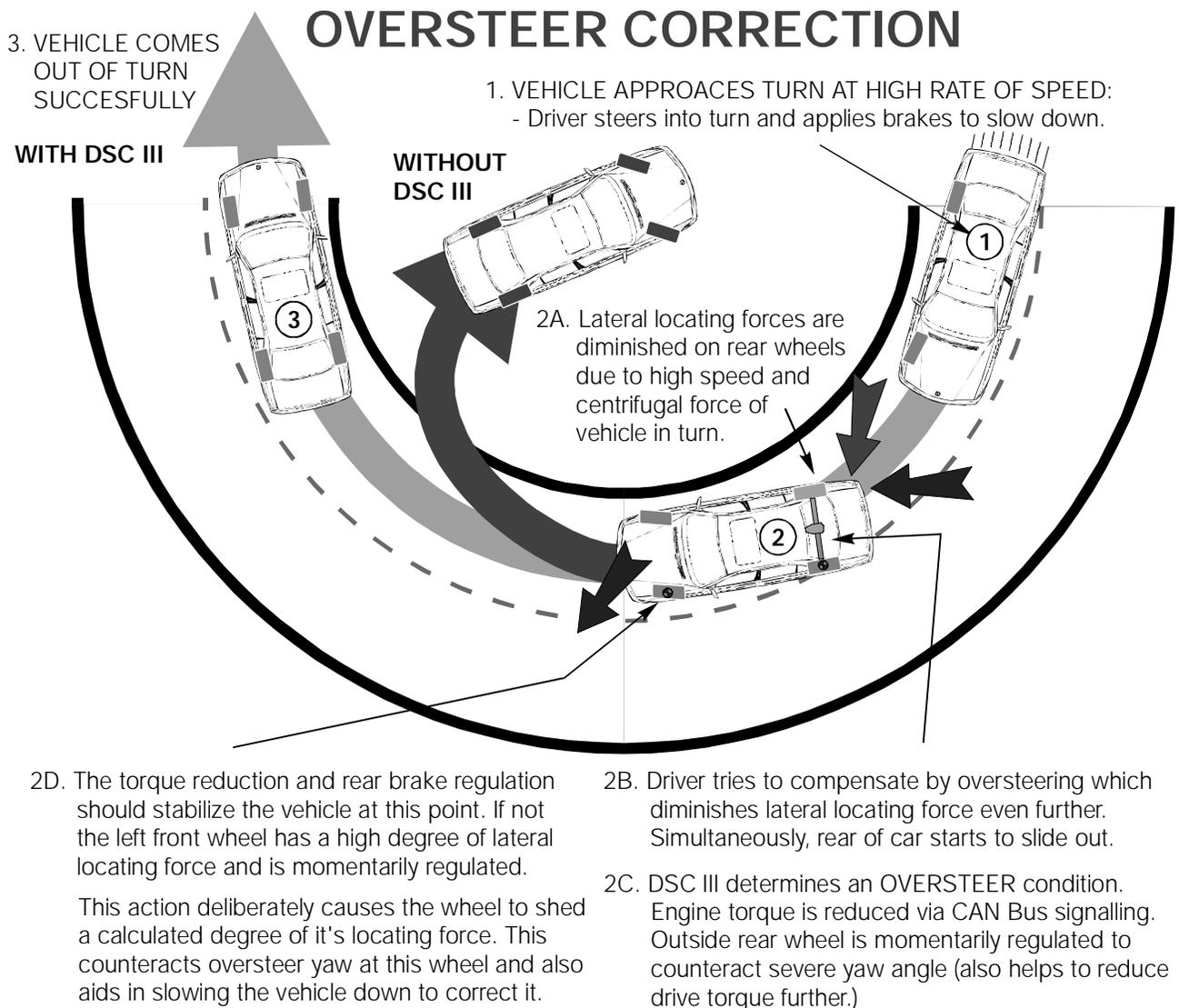
Brake intervention is carried out by the MK60 hydraulic unit if the driver is not actively braking. An example of a brake intervention at the left outside wheel is as follows:
