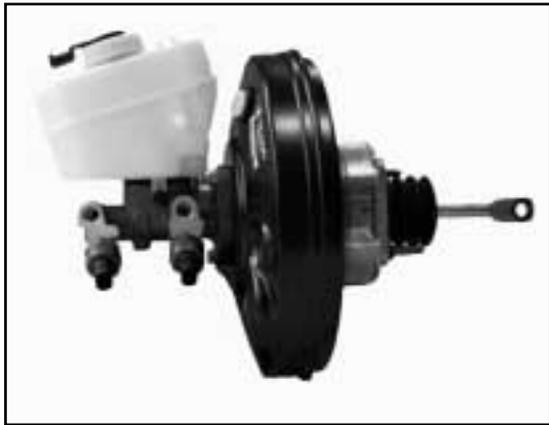
The MK60 system uses a tandem master brake cylinder fitted with central valves as in other DSC master cylinders. The central valves allow fluid to be drawn through the master cylinder during ASC and DSC regulation. The hydraulic circuit is divided front/rear.
