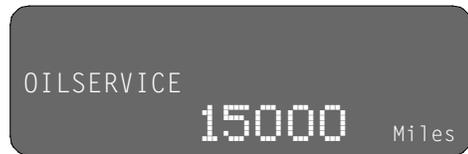
The text "OIL SERVICE" or "INSPECTION" will also illuminate to show which service is due. A minus symbol( - ) before the mileage display indicates that a service is past due.
