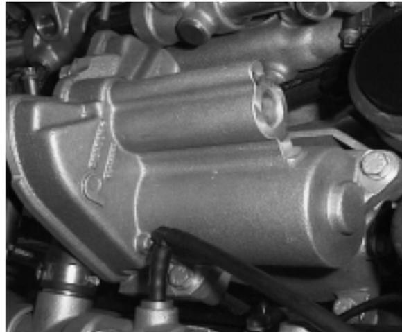
**Idle Speed Actuator:** A separate idle speed actuator (ZWD 5) is used to supply the idle air to all cylinders. The actuator supplies air to the base of the throttle housings which bypasses the throttle valves (plates) to maintain engine idle speed.
