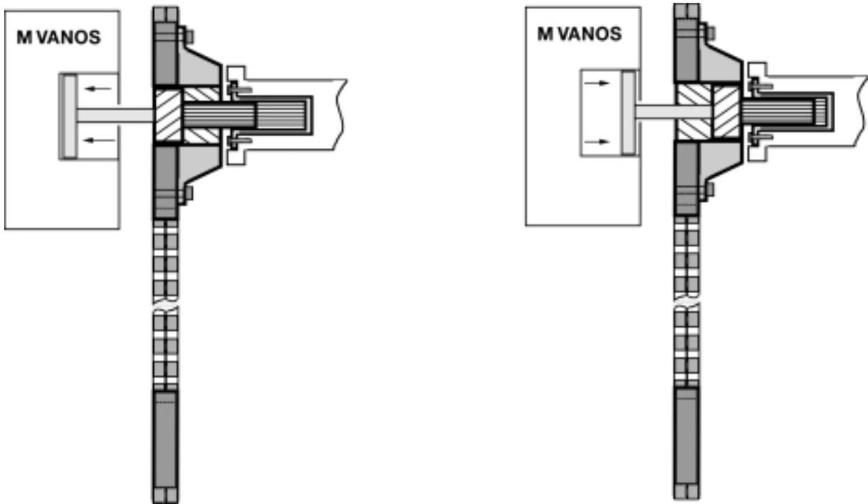
VANOS mechanical operation is dependent on oil pressure applied to position the control pistons. The double VANOS camshafts are infinitely adjustable within the mechanical travel limits of the drive gears.
