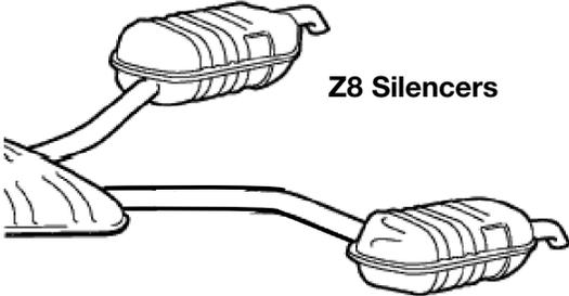
*For repair purposes, the system is separated and sleeved in sections at specific points.*
