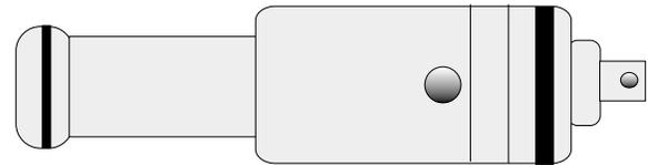
**100 Bar Pressure Regulating Valve:** The 100 Bar pressure regulating valve regulates the pressure produced by the radial piston high pressure oil pumps.
