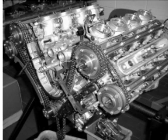
**Camshaft Secondary Drive:** Secondary drive is from the intake camshaft to the exhaust camshaft by a single roller chain (arrow). The chain is tensioned by a hydro-mechanical “self adjusting” tensioner (between the sprockets).
