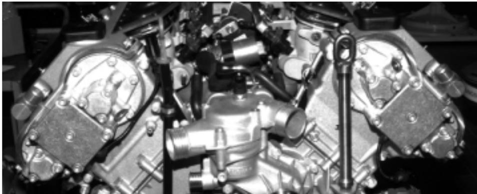
The S62 uses a high pressure (100 Bar) control system that ensures quick and reliable adjustments of the camshafts to meet the high performance requirements of the M Engines. The VANOS units are mounted directly on the front of the cylinder heads.
