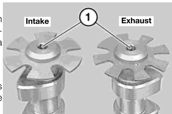
The intake camshaft impulse wheels have 6 lugs and the exhaust camshaft impulse wheels have 7 lugs (including one large lug).
