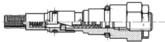
The 100 Bar pressure regulating valve is mounted in the center of the cylinder block “V” on the thermostat housing.
