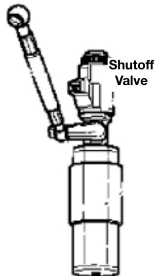
The shutoff valve prevents this because it will close (without electrical power) to reserve a volume of oil under pressure in the accumulator when the ignition is switched off. Upon the next engine start, the valve will be opened by the ECM allowing the stored accumulator release to “prime” the VANOS assemblies with pressurized oil.
