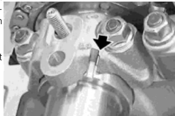
The two grooves should line up to verify correct timing.
