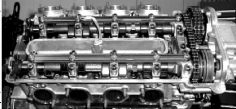
HVA (hydraulic compensators) are used to actuate the valves. ***Valve adjustment is not required.***
