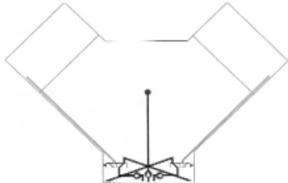
When cornering at forces  $> 0.9g$ , one solenoid will be activated by the ECM to draw oil from the cylinder head while the second solenoid will continue to draw oil from the rear of the pan.
