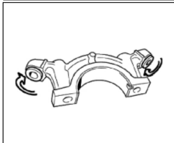
The thrust bearing (#5) is constructed of two radial shells and four shims (example shown on the right).
