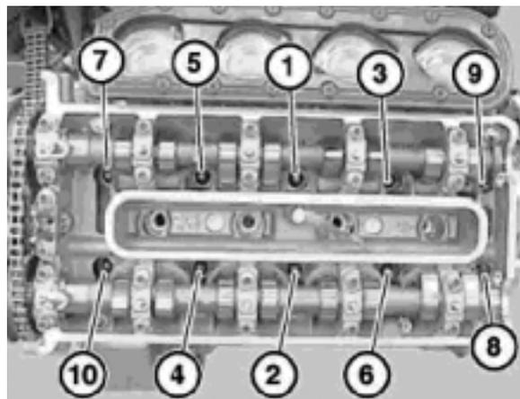
The camshafts are not interchangeable, therefore they should be marked before disassembly.
