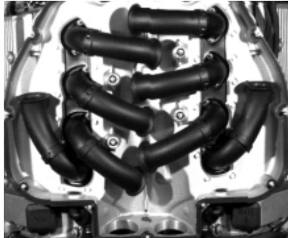
**Intake Air System:** The S62 engine uses eight individual throttle housings that are bolted directly to the cylinder heads. To ensure smooth and stable engine operation all eight throttles must be synchronized for an even distribution of the intake air.
