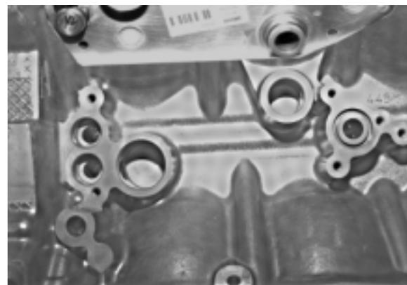
A differential pressure control valve is integrated into the heat exchanger on the oil side. The valve opens an oil bypass in the event that the exchanger should become clogged or at very low start temperatures. This ensures that the engine will receive sufficient lubrication under all driving conditions.
