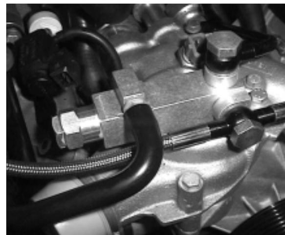
**VANOS Accumulator:** The VANOS accumulator ensures that there is a sufficient volume of oil under pressure to adjust the camshafts under all engine operating conditions.
