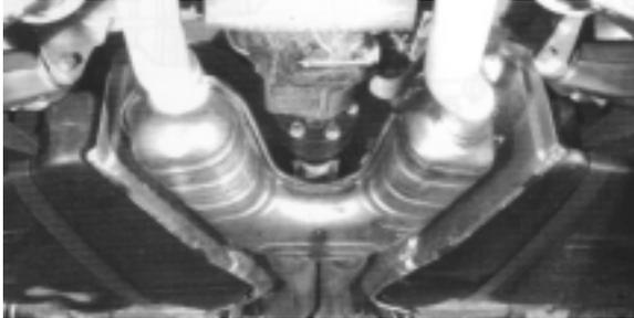
**Main Silencers:** Four main silencers with individual outlets are used on the M5 to comply with international noise emission regulations.
