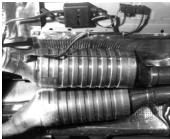
The exhaust is combined in the one piece central silencer with two outlet openings at the rear which lead to the two main silencers.
