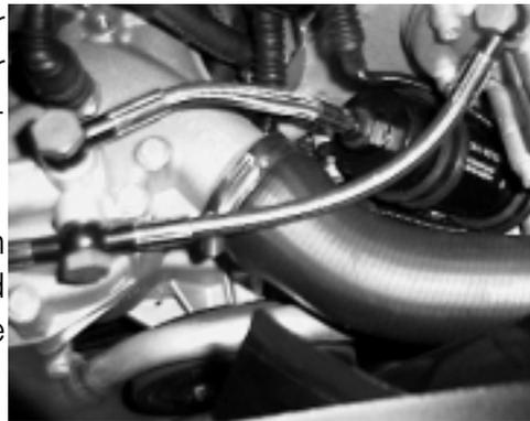
**VANOS Accumulator with Electrical Shutoff Valve:** The VANOS accumulator with an electrical shutoff valve was phased into production on 2001 MY S62 engines.
