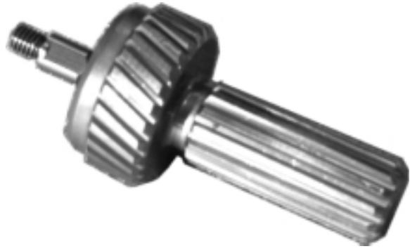
The camshaft sleeves are bolted to the end of the camshafts and engage with the straight spline of the adjustment shaft shown above.
