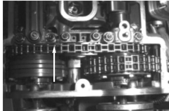
**Camshafts:** The four S62 cast iron overhead camshafts are hollow and are strengthened by heat treating the journals and cam lobes.
