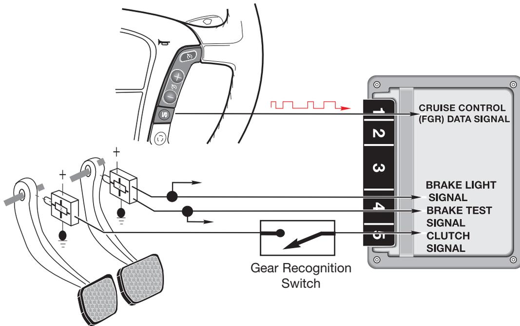
The brake and clutch switch signals are input to the MS S52 control module for cruise control operation.
