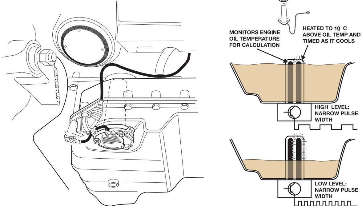
The probe of the level sensor contains two temperature sensing elements.
