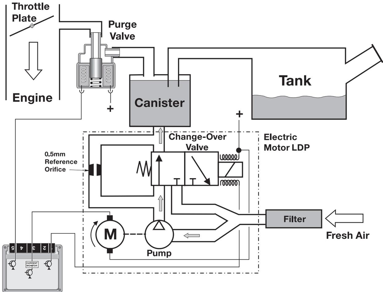
Once the test is concluded, the ECM stops the pump motor and immediately de-energizes the change over valve. This allows the stored pressure to vent through the charcoal canister trapping hydrocarbon vapor and venting air to atmosphere through the filter.
