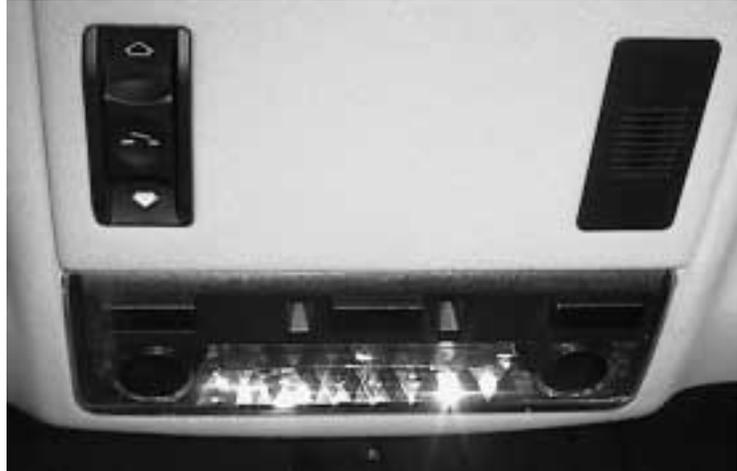
If the switch is held for more than 3 seconds, the GM interprets the continuous ground signal as a request to turn the interior light circuit off for the Workshop Mode as on previous systems. The workshop mode is stored in memory and will not come back on even if the GM is removed from its power supply and reconnected. The switch must be pressed to turn the lights back on.
