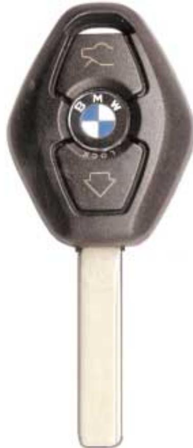
**SERVICE NOTE:** The key memory function of the GM responds to the key identification number of each key. If the keys are not initialized in the same order prior to initialization, the key memory function activated by the keys will not be assigned correctly.
