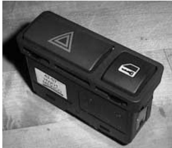
On M.Y. 2000 vehicles, a vehicle that is Double Locked may be opened from inside by pressing the central button once and then manually opening the door from the inside.
