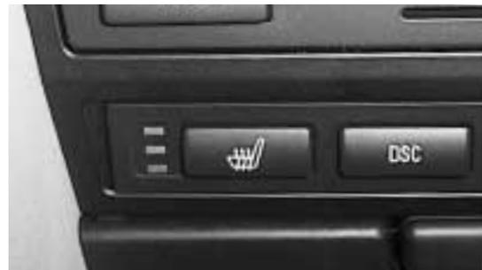
The SZM monitors the seat heating element temperature via an NTC feedback signal to regulate the output current which maintains the seat temperature.
