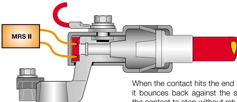
When the contact hits the end stop of the housing it bounces back against the spring tabs causing the contact to stop without returning to the seated position.
