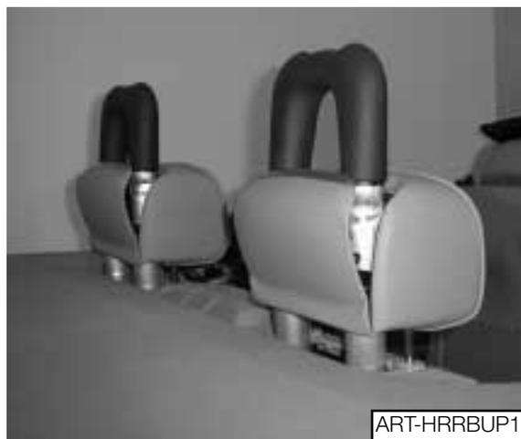
The system is similar to the roll over protection system used on the E36iC. The electronic control module for roll over detection and deployment remains the same as on the E36iC. However, the system has been redesigned in terms of function, solidity and safety.
