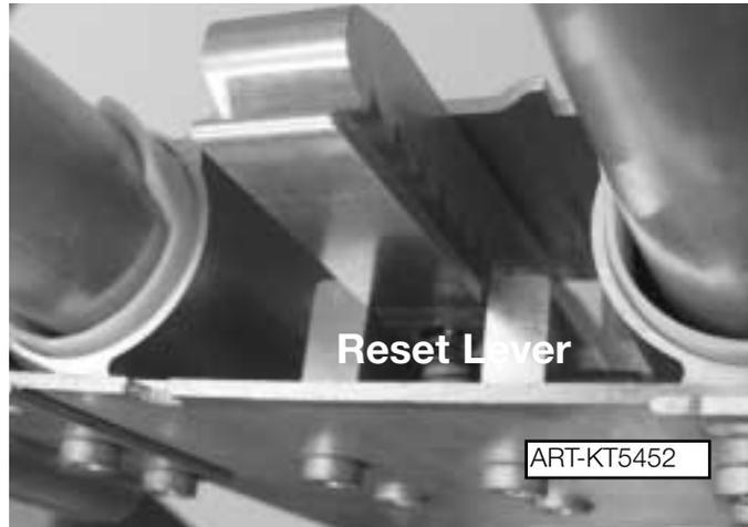
A new resetting procedure is incorporated to retract the bar after deployment. The reset is constructed in the roll bar cassette and the separate tool has been eliminated.
