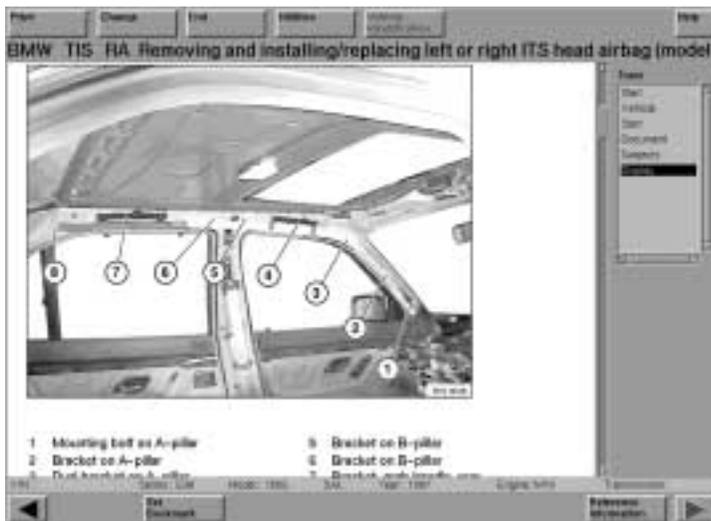
Typical with any airbag, it is to be replaced as a unit after deployment. This is the same for ITS assemblies and the BST.
