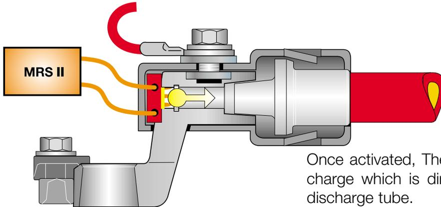
Once activated, The ignitor generates a gas charge which is directed down the internal discharge tube.
