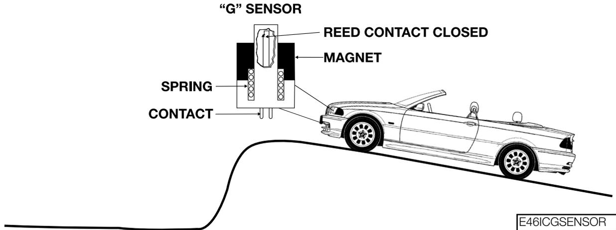
However, if the vehicle becomes airborne and weightlessness occurs, the spring will force the magnet up and the reed contact will open. This will signal the electronics of the sensor to trigger the solenoids and the roll bar will deploy.
