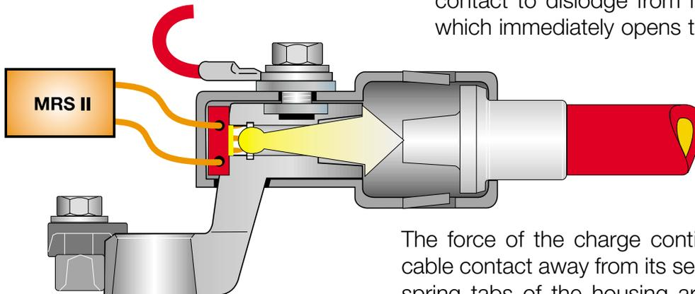
The force of the charge continues to push the cable contact away from its seated contact. The spring tabs of the housing are compressed as the contact pushes to the end of its travel.
