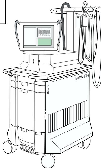
**Test Modules:** Faults with the E46 IHKR can be diagnosed using fault or symptom driven test modules. To begin diagnosis:
