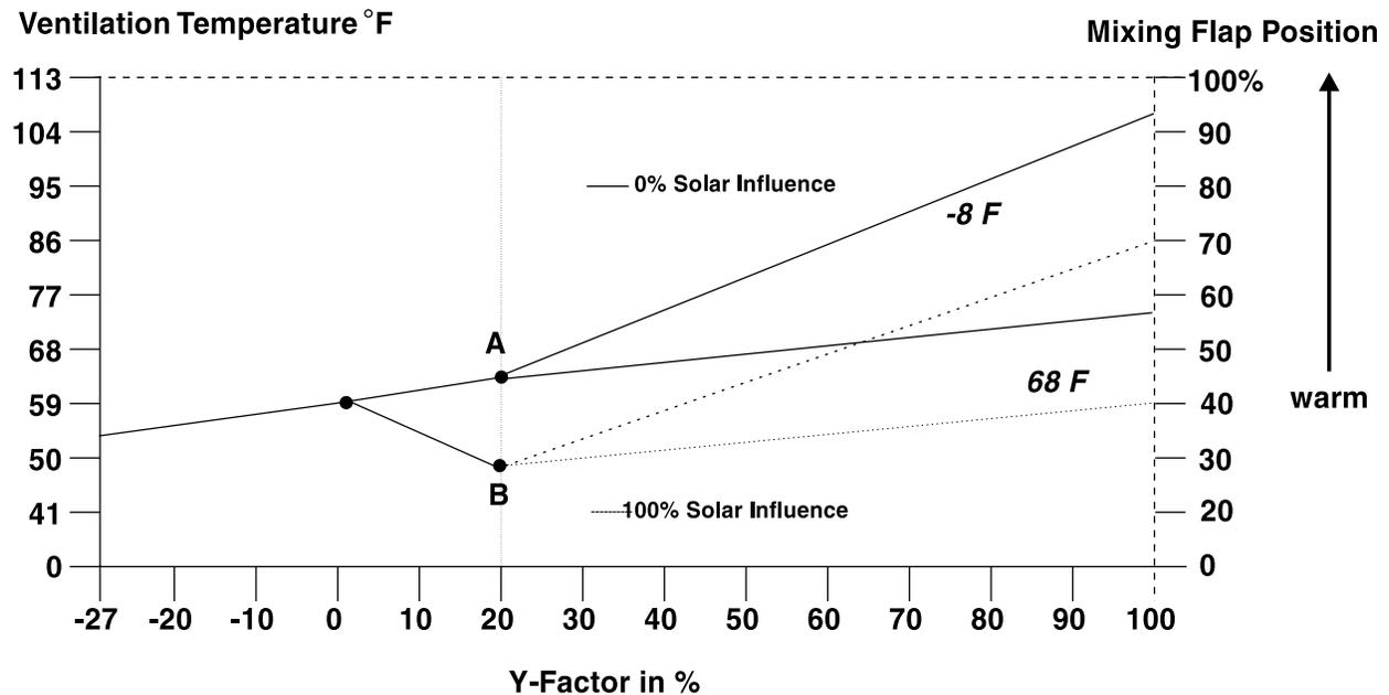
To illustrate the influence of the solar sensor on the mixing flap position, the Y factor remains constant at 20%.
