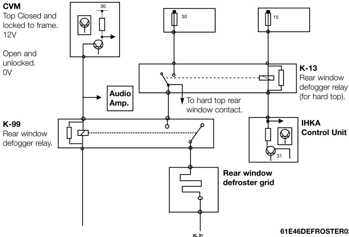
Relay K-13 also supplies KL 30 to relay K-99 when the button is pressed on the IHKA control panel. Relay K-99 is energized when KL R is switched ON and the soft top is closed and locked to the windshield frame. This allows the grid in the soft top window to be heated. When the soft top is lowered, KL R to relay K-99 is interrupted by the CVM to prevent the grid from heating when the top is lowered into the storage compartment.
