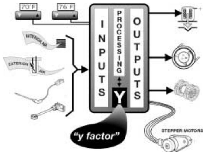
The processed variable "Y-factor" is determined by using the above inputs. The Y-factor then represents how much adjustment is necessary by the IHKA module to achieve the set temperature.
