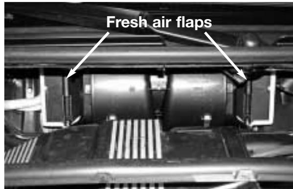
When the key is turned off with re-circulation on, the fresh air flaps will open. Re-circulation memory in the IHKR control unit is 15 minutes. If the vehicle is started within 15 minutes the re-circulation setting will be restored.
