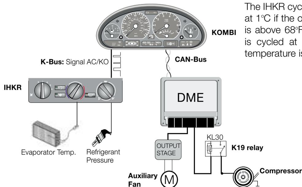
The IHKR cycles the compressor at 1°C if the outside temperature is above 68°F. The compressor is cycled at 3°C if the outside temperature is below 68°F.
