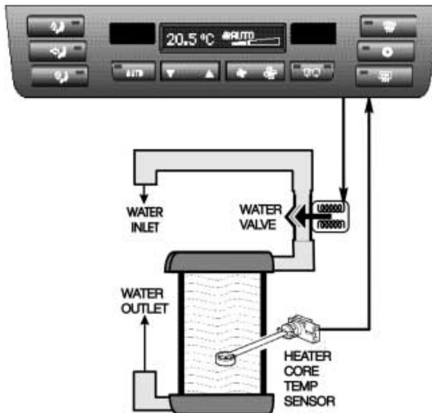
**SERVICE STATION FEATURE** - The "Service Station" feature introduced with the E38 IHKA is integrated into the E46 IHKA. This prevents the heater core from being flooded with hot coolant when refueling the vehicle.
