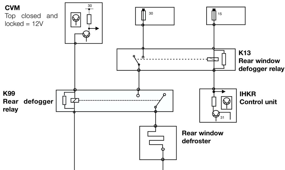
When the button is pressed on the IHKR control panel, relay K13 is energized. K13 supplies KL 30 to defroster relay K99. Relay K99 is energized when the KLR is switched on and the soft top is closed and locked to the windshield frame. This completes the circuit and allows the rear window to be heated.
