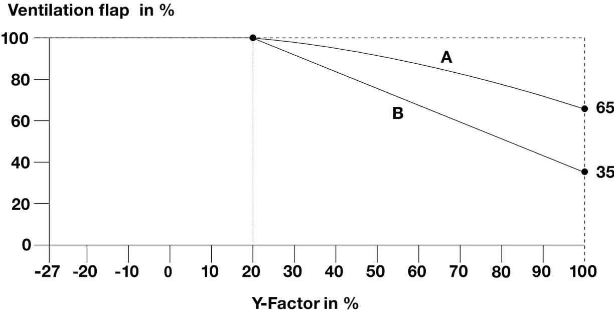
The normal curve “B” applies when there is no solar sensor influence 0%, or if the sensor is defective.
