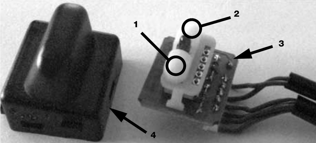
**DWA LED dismantled; housing and pc-board with LED and solar sensor housing**
