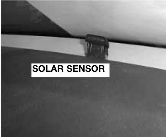
The E46 solar sensor is located in the right defroster outlet at the base of the windshield. The E46 sensor contains one photoresistor for sensing solar radiation.
